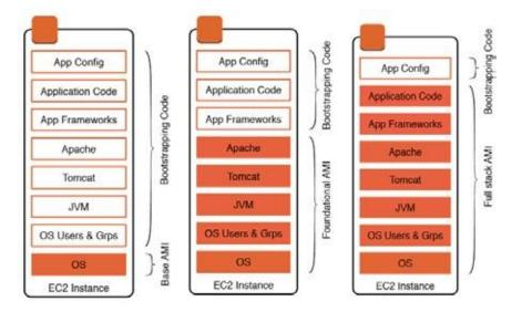
Figure 3: Differences Between Fully-Cconfigured and Base AMIs
